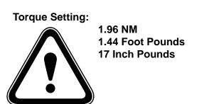
DO NOT OVERTIGHTEN OR YOU COULD RESTRICT THE OIL FLOW VERIFY COMPRESSOR LOADS UP
